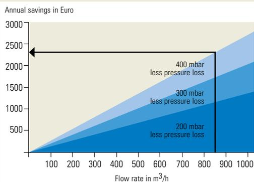
A decrease of differential pressure by only 400 mbar saves 2,300 EUR per year. (with 8,000 operating hours/year, 7 bar mains system pressure, 90 kW installed capacity and 0.08 Euro/kWh)
